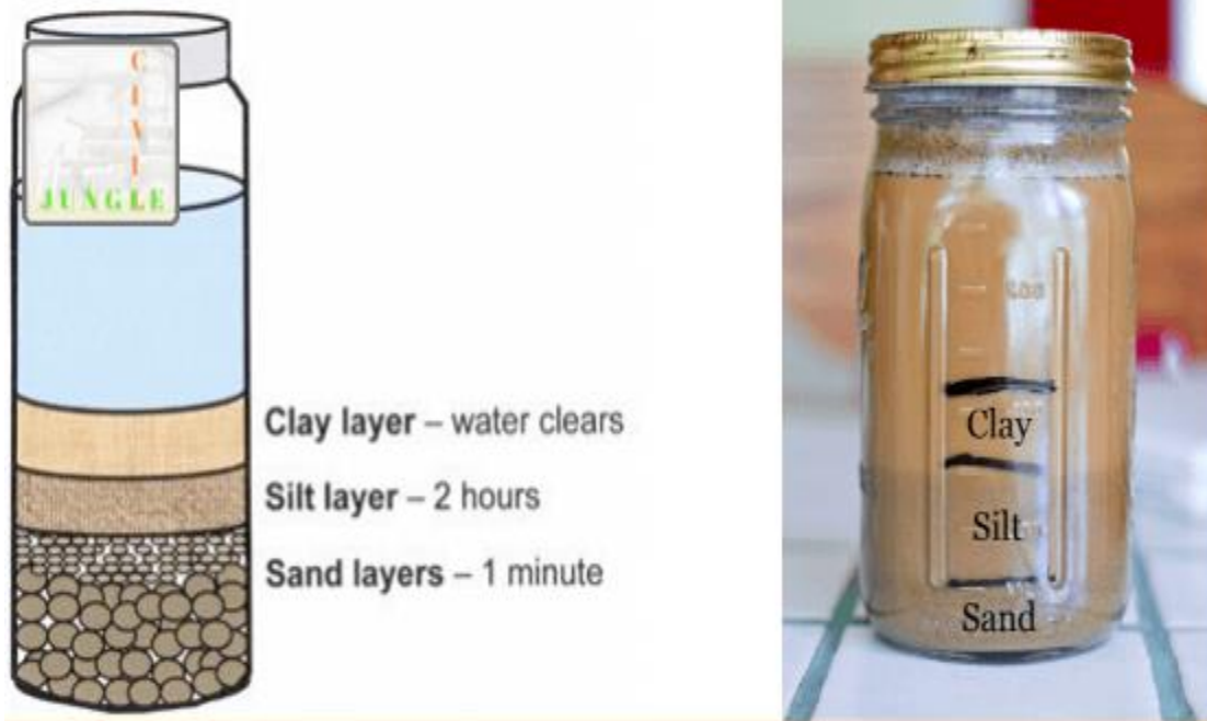
Figure 25 Testing for Silt Content in Sand
