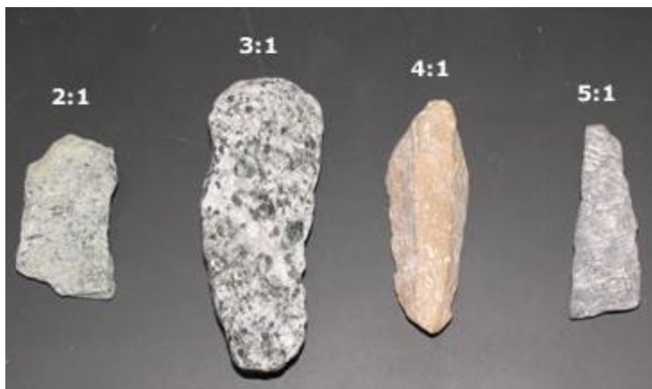
Figure 20 Sizes of Flat and Elongated Particles
