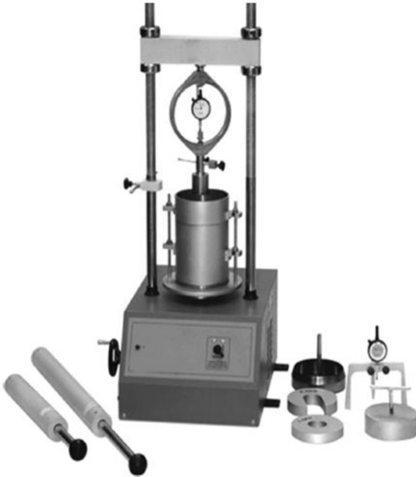
Figure 32 CBR Test Equipment and its Accessories
